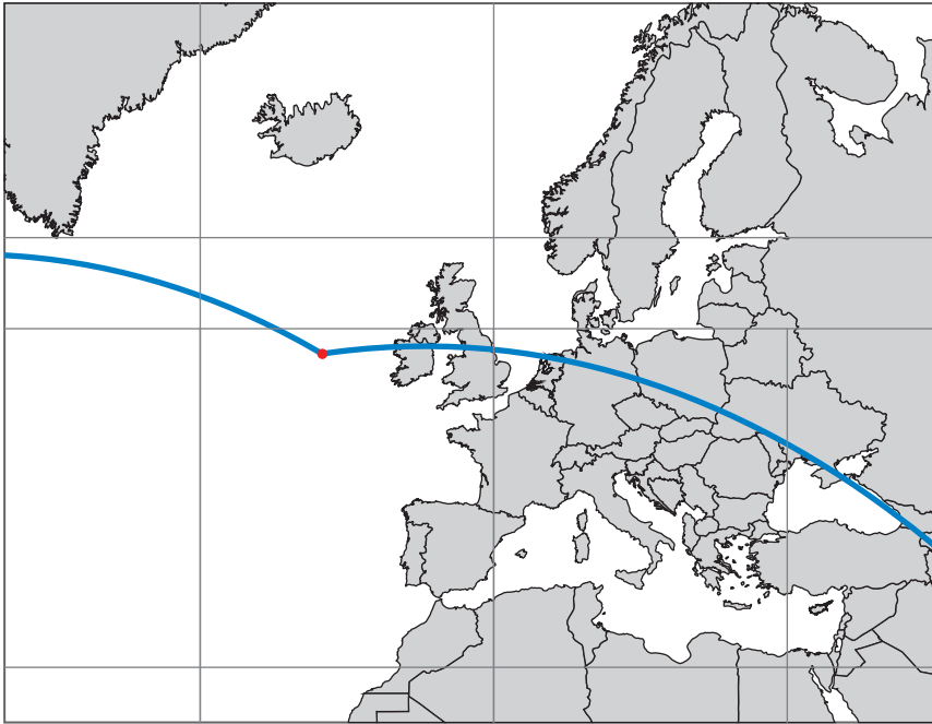
Figure 4.4 Apogee Plane Change to Avoid Overflight of Russia
