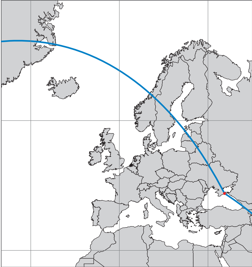
Figure 4.2 Illustrative Minimum Angle Plane Change to Avoid Overflight of Russia
